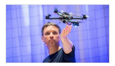
Mini-robots are rapidly improved as well. This one receives its energy from a nearby laser and hence does not need a heavy battery.
